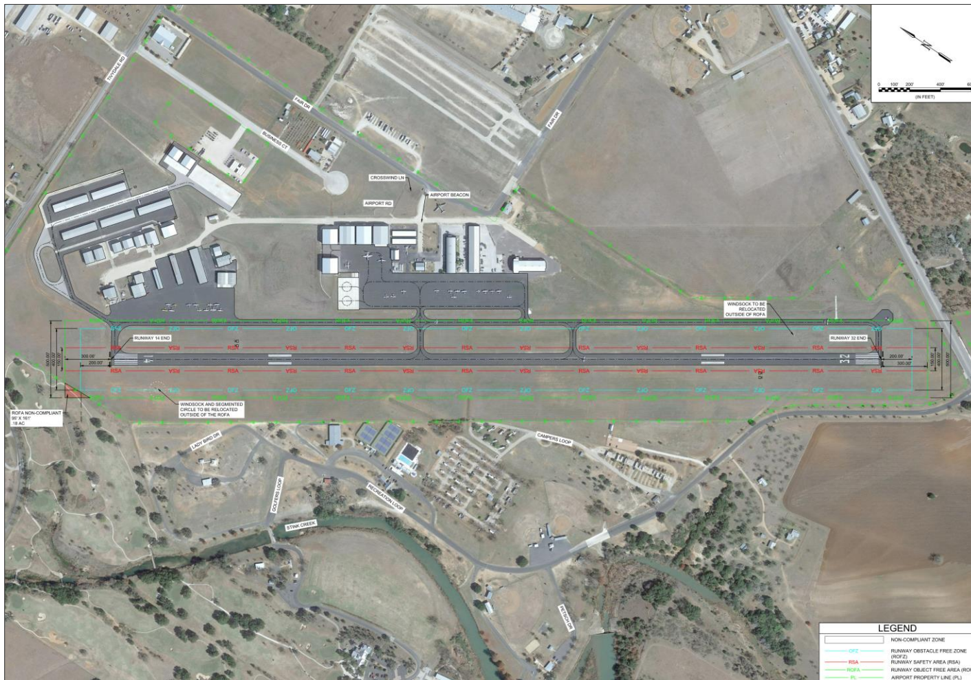
FIGURE 4-2 RUNWAY 14/32 ROFA DEFICIENCIES GILLESPIE COUNTY AIRPORT
